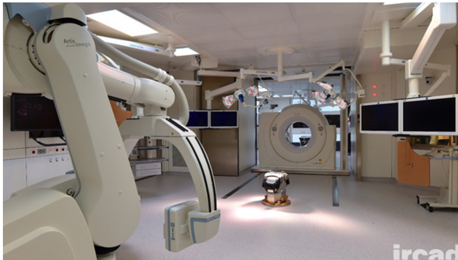
Figure 1 IHU-Strasbourg hybrid room for image-guided procedures. The hybrid operating room (OR) at IHU-Strasbourg integrates (I) a robotic multi-axis 3D angiographic system (Artis Zeego, Siemens Healthcare, Erlangen; Germany); (II) a CT-scan, which is mounted over rails and can be “called in”, when required, in a matter of seconds; and (III) an MRI room with the door which opens in the OR (not shown).
