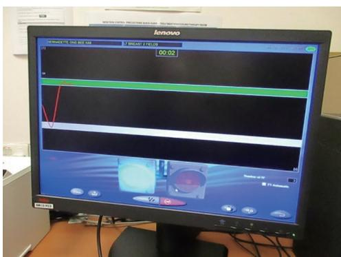
**Figure 2** SDX Spirometric Gating System. Green bar shows the breath hold region where radiation will be delivered.
