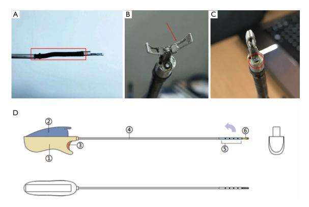
Figure 1 The structure of visual multifunctional blunt separator. (A) The flexible joint (dotted box) in the distal; (B) the blunt separation head (arrow); (C) the camera (dotted circle) in the distal; (D) the appearance of the instrument: 1 handle; 2 key (control the bend of flexible joint); 3 trigger (control the opening and closing of blunt head); 4 metal rod; 5 the flexible joint; 6 the blunt separation head.
