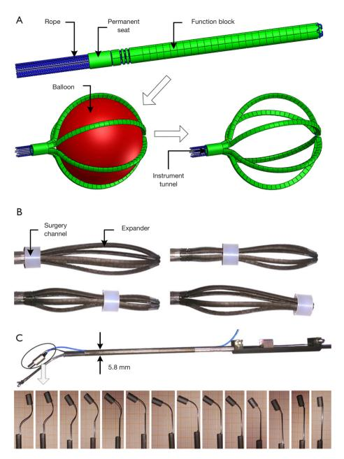
Figure 3 Working procedure of the dilator and operating system. (A) Working process of the dilator; (B) procedure of the dilator removed from the surgical channel; (C) swing process of the lens mount.
