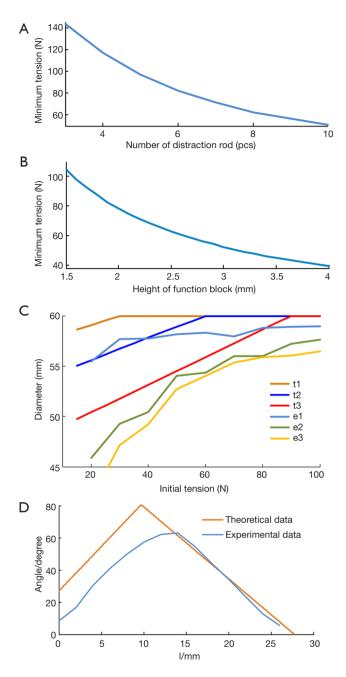
**Figure 4** Result of analysis of the dilator and the operating system: (A) the minimum tension under the different number of identical unit; (B) the minimum tension at different height of identical unit; (C) analysis and experimental result of the diameter of the dilator under different initial tension and loading; (D) kinematics analysis and experimental result of the operating system.
