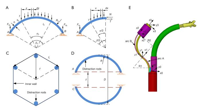
**Figure 2** Schematic diagram of force analysis of the dilator: (A) the analysis of force on identical unit; (B) the force analysis of half identical unit; (C) the simplified relationship between the identical unit and the inner wall of uterus; (D) the schematic to get the diameter of the dilator; (E) the schematic of kinematics analysis of the operating system.
