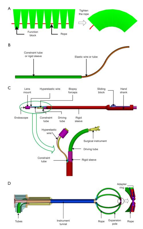
**Figure 1** The working principle and structure of the mechanical dilatation device: (A) working principle of the dilator; (B) hyperelastic wire and tube structure; (C) structure of the operating system; (D) structure of the dilator.
