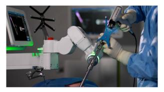
**Figure 5** Mazor X stealth edition navigation DRB (Black 6 marker array) and navigated instrument (Blue 4 marker array).
