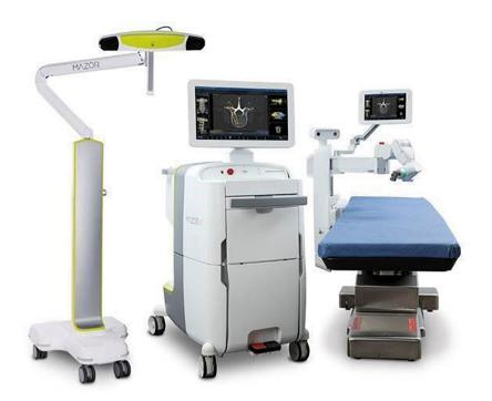
Figure 4 Mazor X stealth edition platform. Navigation tracking camera (left), base station (middle), bed (and patient) mounted robotic arm with end effector (right).
