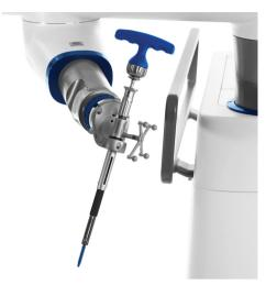
Figure 3 Globus Excelsius GPS end effector with navigated instrument.
