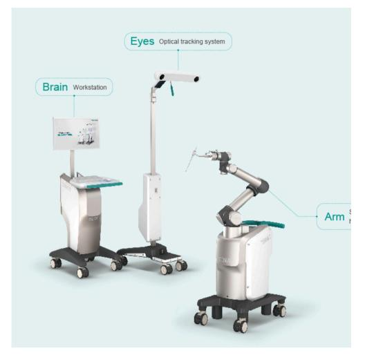
Figure 6 TINAVI TiRobot platform. Base station (left), optical tracking camera (middle), and floor-mounted robotic arm (right).
