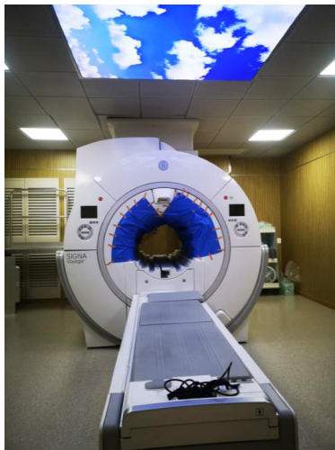
Figure 4 The entire inside wall of the magnet hole was stuck by the two-layer disposable hospital bed sheets to prevent the potential contamination caused by the patient's cough droplets during scanning.
