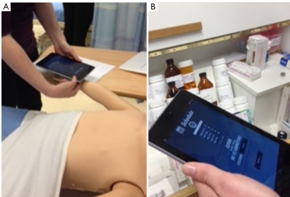
Figure 3 NFC system testing. (A) Scanning NFC tagged patient bracelet; (B) medication administration using NFC system.
