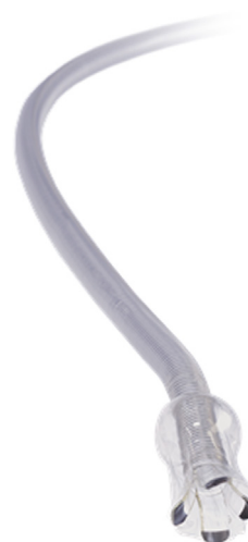
Figure 10 AngioVac aspiration cannula with coil-reinforced body to prevent collapse during application of negative pressure and balloon-expandable tip to maximize thrombus engagement and removal.
