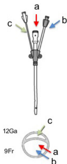
Figure 1 The arrow multilumen access catheter. The lumen a and b together have a diameter of 9 Fr, and the lumen c independently have a diameter of 12 Ga.
