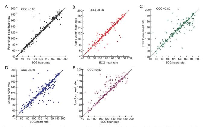
Figure 2 CCCs depicting agreement of device-measured HR with ECG. (A) Polar H7; (B) Apple Watch III; (C) Fitbit Iconic; (D) Garmin Vivosmart HR; (E) Tom Tom Spark 3. CCC, concordance correlation coefficient; HR, heart rate.
