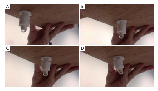
Figure 1 Wireless steerable endoscope (WSE) prototype. The WSE is held against gravity by a magnet under a wooden plank mimicking attachment to the internal wall of a body cavity (A). The WSE can (B) slide; (C) axially rotate; (D) providing multiple viewing directions [Reprinted with permission (8)].
