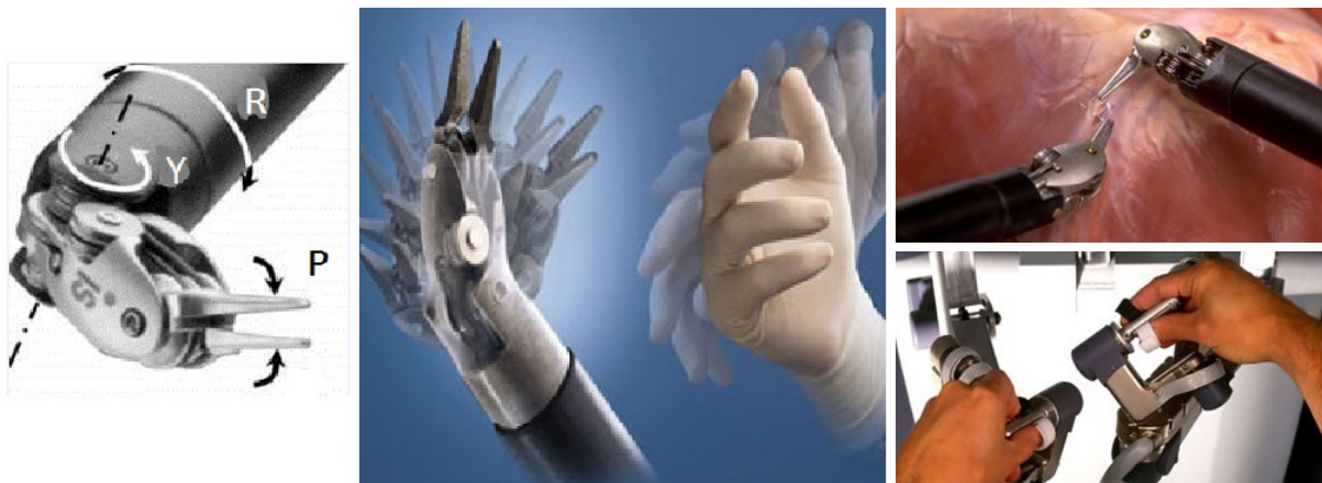
Figure 2 da Vinci system’s EndoWrist instruments.
