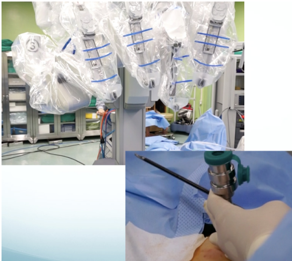
Figure 6 The angle for docking of robot. The robot cart is docked obliquely along the imaginary line from the camera port to the anterior superior iliac spine.
