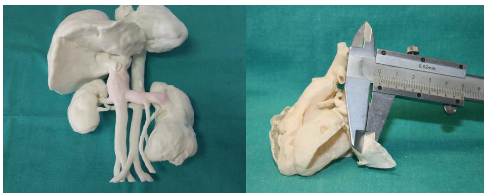
Figure 1 Renal tumor and thrombus in cava vein model (0.8 mm wall thickness) and congenital heart disease model (0.4 mm wall thickness).
