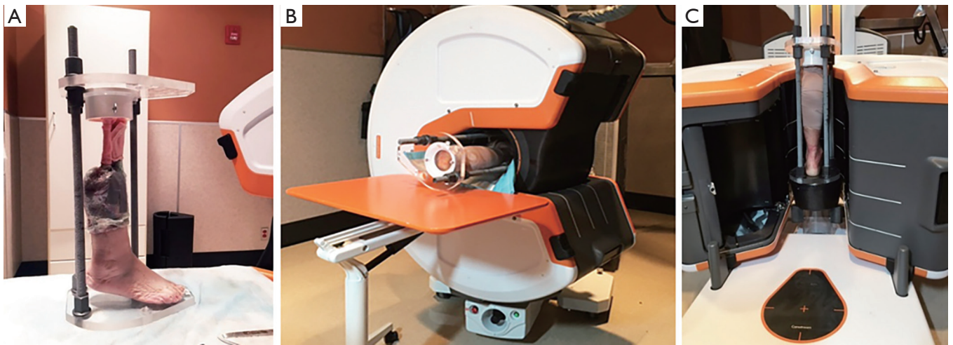
Figure 1 Illustration of experimental testing set up. (A) The testing rig consisted of Plexiglas top and base, each milled to the shape of the cone-beam computed tomography (CBCT) scanner's foot plate. (B) An ankle specimen in the CBCT scanner positioned for a gravity stress scan. (C) An ankle specimen in the CBCT scanner positioned for a weight-bearing scan after 222 N load was simulated.
