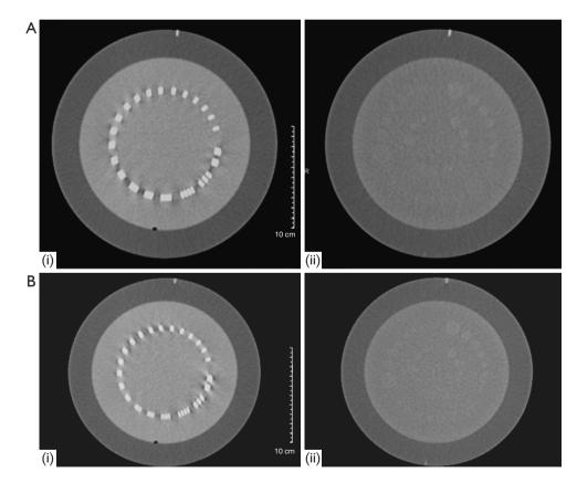
**Figure 1** Phantom images demonstrating image quality in the standard protocol (120 kV/90 mAs) (A) and the low dose protocol (100 kV/115 mAs) (B). This is no significant difference in the spatial (i) and contrast resolution (ii) between these two protocols. kV, kilovoltage.
