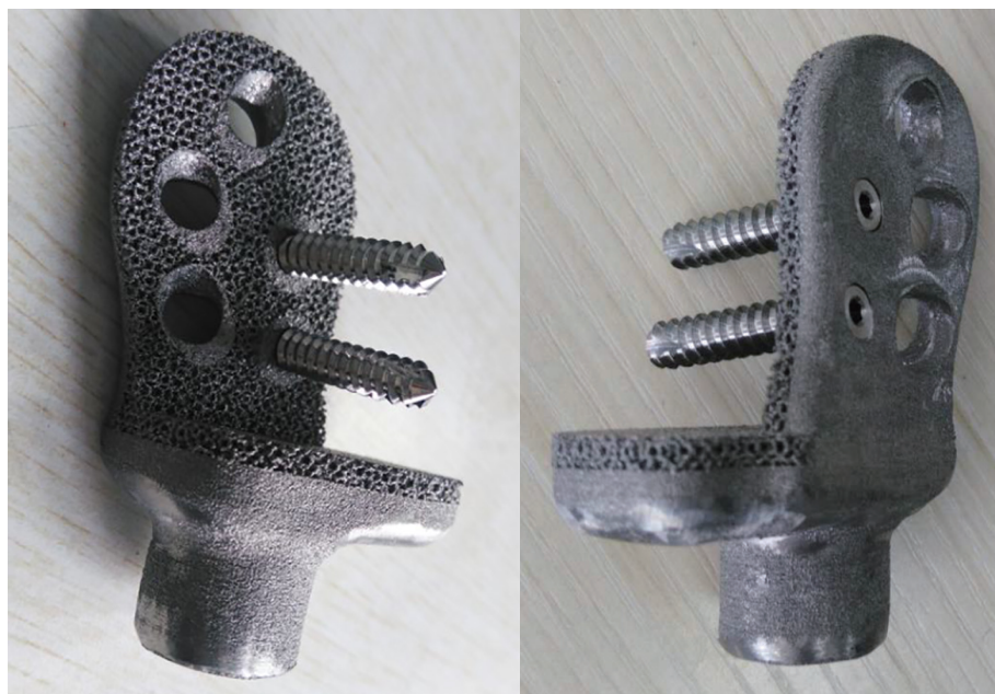
Figure 2 The second generation of modular hemipelvic endoprosthesis manufactured by EBM. EBM, electron beam melting.
