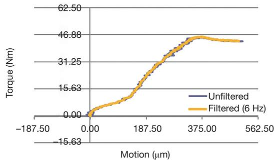
**Figure 4** Torque (Nm) *vs.* relative motion ( $\mu\text{m}$ ) between implant and distal femur.
