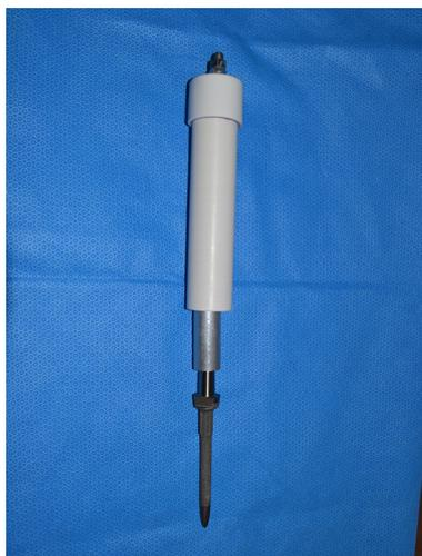
**Figure 2** Spring-based insertion tool designed to fit over standard Stryker inserter and calibrated to standard force of 50 N (60 lbs.)
