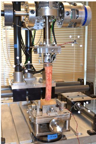
**Figure 3** Potted and implanted specimen in torsional testing apparatus (i.e., on a multi-axis biomechanical test frame with Vicon 3-D motion analysis reflective infrared targets attached).
