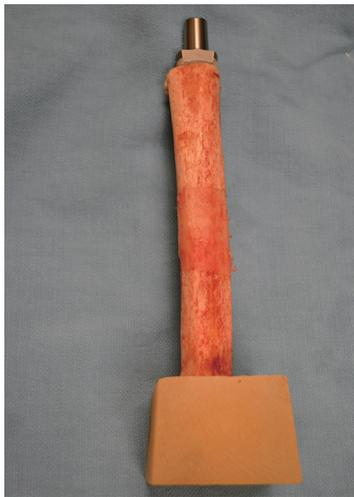
**Figure 1** Potted femoral specimen with implanted stem.
