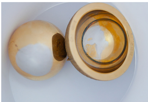
Figure 5 Retrieved ACCIS acetabular and femoral component showing the wear patch on the head and cup surfaces (courtesy of K De Smet).
