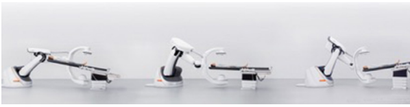
Figure 1 Artis pheno is robotic C-arm by Siemens, able to position in many different dimensions based on the patient, procedure, condition and operator needs. (Image courtesy: Siemens)
