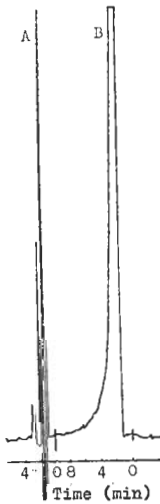
Fig 3. Chromatograms of \text{HClO}_4 0.05 mol/L, containing 0.1% EDTA (A), and 0.1% EDTA + 0.1% \text{Na}_2\text{S}_2\text{O}_5 (B). Column, LiChrosorb RP-18, 5\mu\text{m} ( 15 \times 0.5 cm, ID); mobile phase, \text{KH}_2\text{PO}_4 0.1 mol/L, EDTA 0.1 mmol/L, CSA 9 mmol/L (pH 3.5) and 6% \text{CH}_3\text{OH} .
