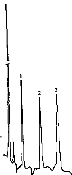
Fig 1. Chromatogram of control plasma spiked with 500 ng · ml -1 nifedipine (peak 1, Rt 6.13 min) and internal standard (peak 2, Rt 8.94 min) and m -nifedipine (peak 3, Rt 11.37 min)
