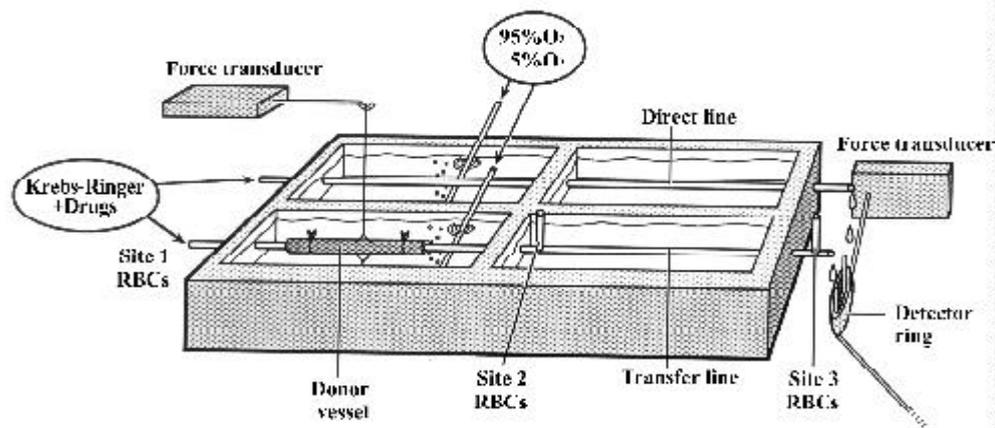
Fig 1. Schematic representation of the used perfusion-superfusion bioassay system.
