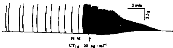
Fig 3. Effect of CT-14 on isolated rat phrenic nerve-diaphragm. Twitches were elicited by electric stimulation on nerve (N) or diaphragm (M) with supermaximal voltage (90 V), 0.1 Hz, and 0.5 ms pulse duration.
