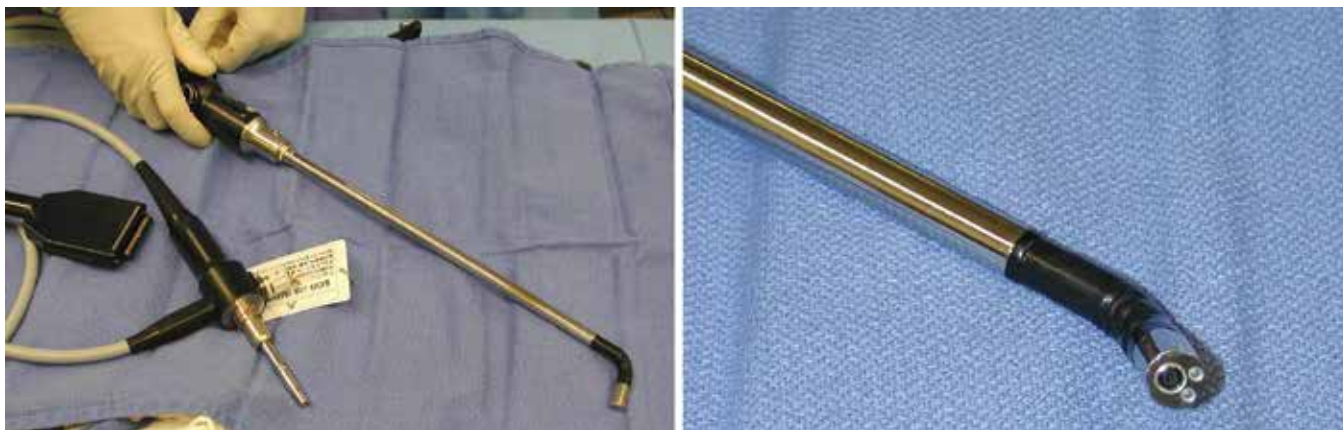
Figure 1 High definition, thoracoscopic video camera with deflectable tip. (Olympus Surgical and Industrial America Inc., Center Valley, PA).
