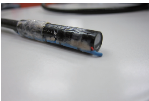
Figure 3 The Aldiscope. A fine bore infant feeding tube has been wrapped around the borescope to act as a port for irrigation.
