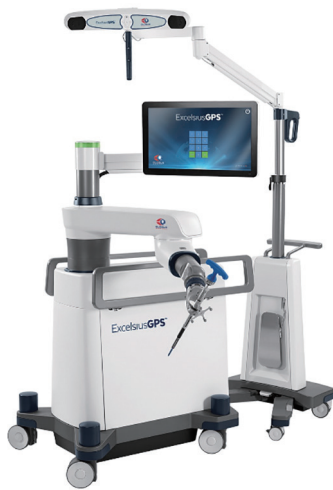
Figure 1 The ExcelsiusGPS surgical system (Globus Medical, Inc., Audubon, PA, USA). This system guides pedicle screw insertion via a patient-mounted reference array.
