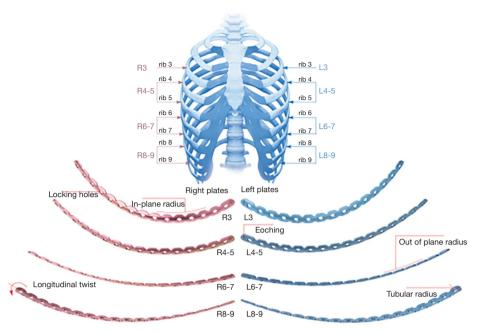
Figure 1 An example of a rib plating system (39). Note that the plates are contoured for specific ribs, including laterality. *Courtesy of DuPuy Synthes* (© *DePuy Synthes 2017*).
