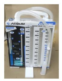
**Figure 1** The analog drainage system Ocean Atrium (Maquet, Germany): a classical wet-seal drainage system with an analog scale to measure the total amount of fluid, a surge chamber and external vacuum-suction.
