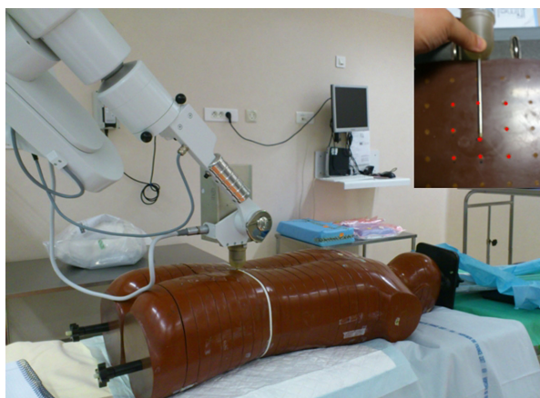
Figure 1 Set-up of a Kypho-IORT treatment using an anthropomorphic phantom with thermoluminescent dosimeters (TLD) positioning inside the phantom and on the skin. IORT, intraoperative radiotherapy.
