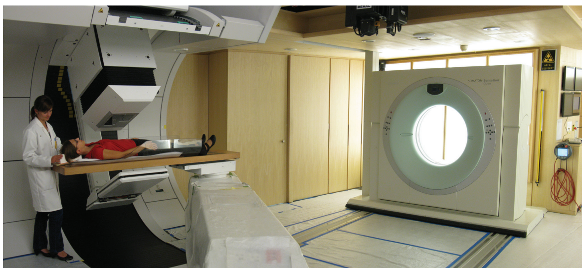
Figure 3 Photograph of Gantry 2 treatment room with gantry-angle set to +20^\circ . Visible on the left are the patient-table, the false fixed floor around the patient-table for easy access to the patient, the extractable nozzle, the rolling cover where the nozzle rotates and the BEV. Note that the BEV is extracted with the imager positioned along the proton beam direction just downstream from the patient. Noteworthy on the right is the sliding-CT, with the rails clearly visible on the floor. A white protective film is currently covering the floor and patient-table prior to treatment of first patient
