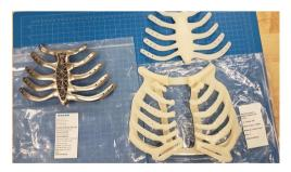
**Figure 4** Titanium prosthesis (left), plastic reconstructions for preoperative planning (right).
