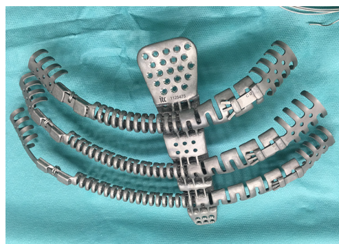
Figure 12 Titanium 3D printed implant with biomechanic design.
