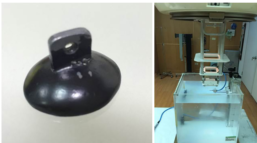
Figure 1 Eye shield (left) and water phantom (right).
