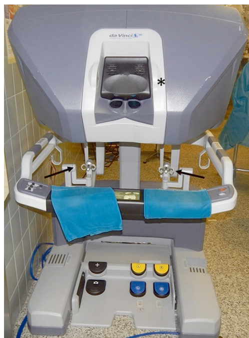
Figure 4 Close look to the surgeon's console: binocular (*), master controls (arrows), buttons and pedals.
