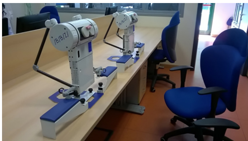
Figure 3 A compact, lightweight and portable system of robot-assisted surgery simulator, “Actaeon”, developed by BBZ, a spinoff company from the University of Verona (Italy).
