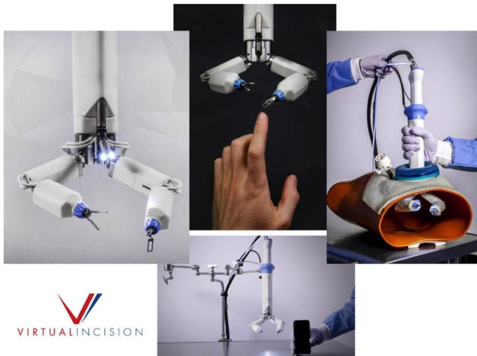
**Figure 9** Miniature *in vivo* robots. The Virtual Incision surgical robot is shown (Virtual Incision, Omaha, NE, USA). Reproduced with permission from (14).
