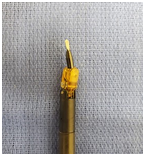
Figure 5 Spatula for use in the da Vinci robotic system. Robotic spatula works by causing superficial tissue desiccation over a wide area.
