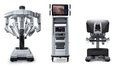
Figure 1 The da Vinci Xi<sup>®</sup> robotic surgical system—a sample view of the robotic operating console, surgical robotic, and surgical monitor. (Intuitive, Incorporated; Sunnyvale, CA).
