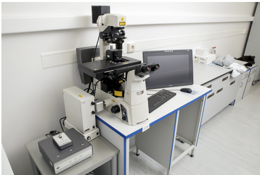
Figure 2: Example of laser capture microdissection workstation (11).
