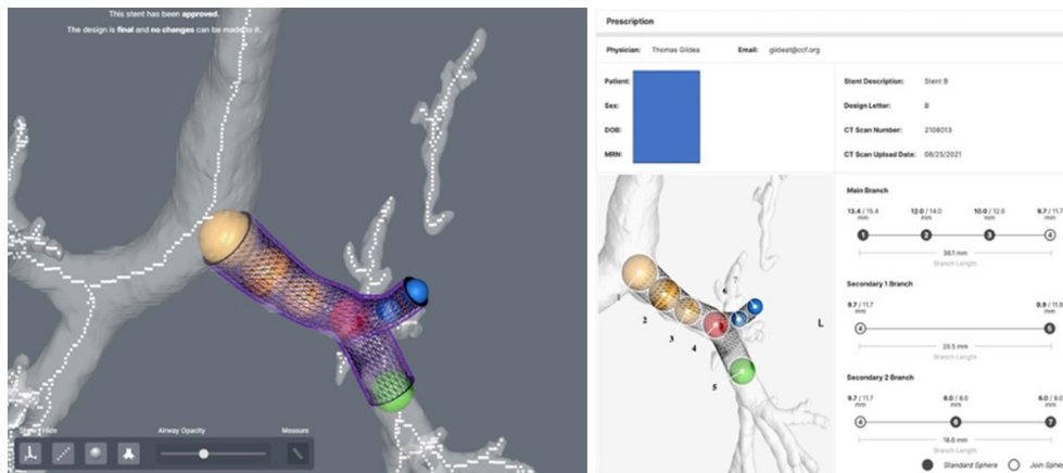
Figure 1 After a 3D virtual prototype of the airway is created. The physician uses the software tools to place a series of spheres in the desired area to adjust the shapes and sizes to make a virtual representation of the patient specific silicone stent based on clinical needs. Picture authorized by COS Inc., Cleveland, OH, USA (Visionair). 3D, three-dimensional.
