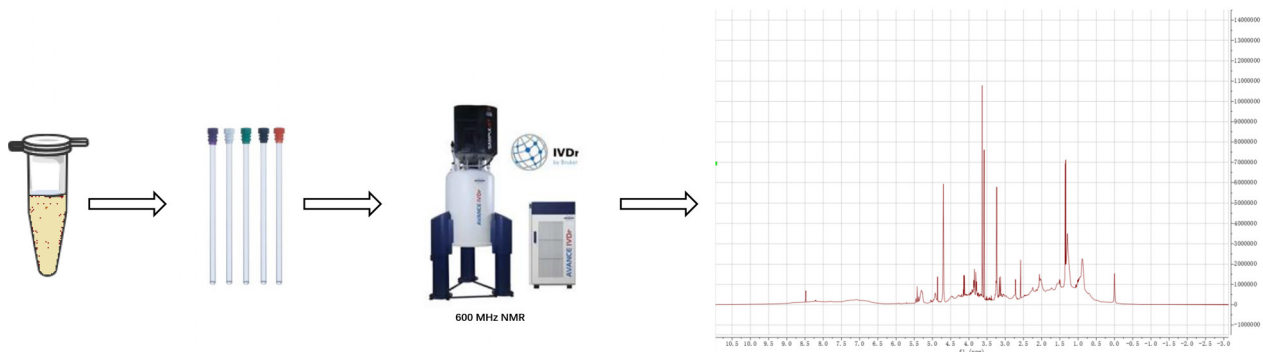
Figure S1 Flowchart of metabolomics detection. The patient's plasma was transferred to the NMR tube and placed in a 600-MHz NMR instrument for detection, and the H-1 spectrum data were obtained for analysis. NMR, nuclear magnetic resonance.
