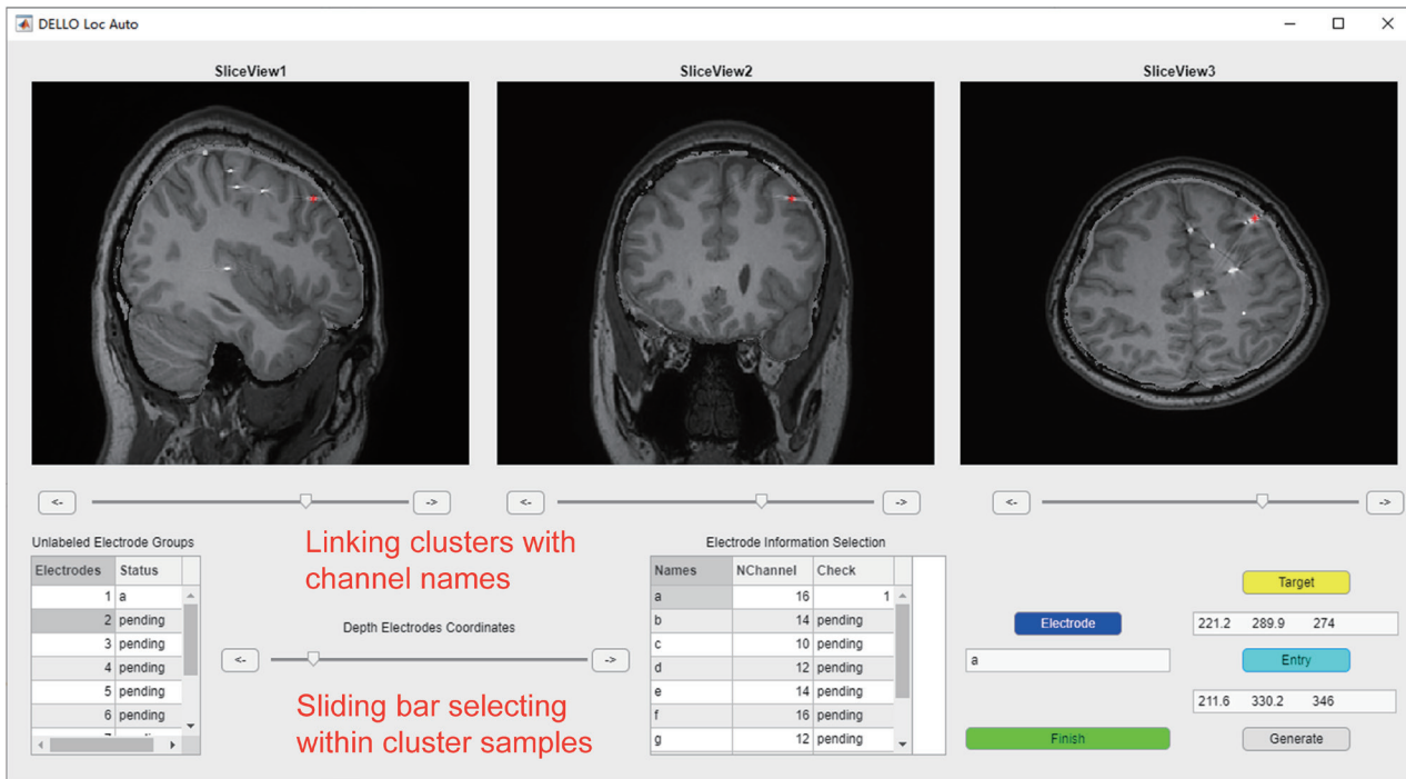
Figure 5 Electrode naming panel. Users should select the matched cluster groups and the electrode name cells to rename the specific electrode shaft. The sliding bar is used to select samples within 1 electrode shaft and define the target and entry points. The coordinates of each contact are calculated.
