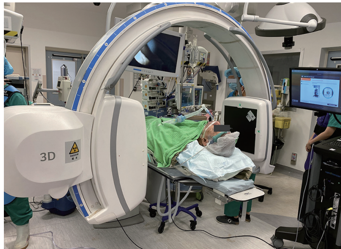
Figure 3 This figure shows the operating room setup during Cios Spin® mobile C-arm image acquisition.
