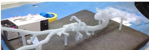
**Figure 4** Post production finishing including removal of the supporting structures and application of an ultraviolet (UV) light resistant polish/varnish.
