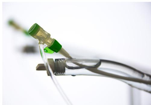
**Figure 7** 6-Fr sheath inserted into the model through the pre-designed access site.
