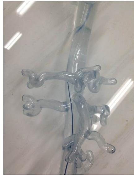
**Figure 5** Following application of the polish the material has a transparent result.
