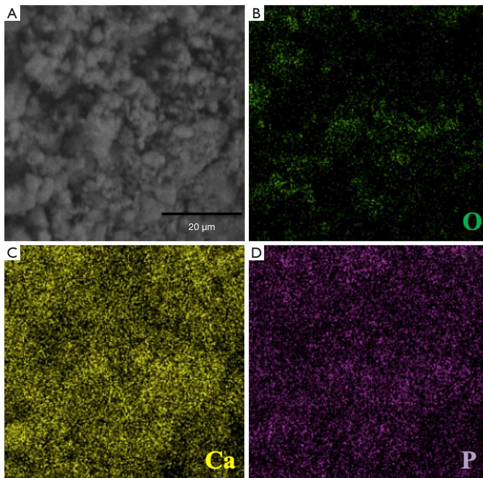
**Figure 3** EDS elemental mapping of the  $\text{Ca}^{2+}/\text{PO}_4^{3-}$ @MSN complex. (A) Image of  $\text{Ca}^{2+}/\text{PO}_4^{3-}$ @MSNs, (B) EDS O elemental map, (C) EDS Ca elemental map, (D) EDS P elemental map. The elements of Ca, P, O were evenly distributed. EDS, energy dispersive spectrometer; MSNs, mesoporous silica nanoparticles.
