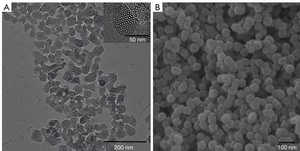
**Figure 1** TEM (A) and SEM (B) images of MSNs. MSNs exhibit even particle size and nearly spherical structure with a diameter of approximately 50 nm. The distribution of the inner core is also even and similar in size. TEM, transmission electron microscopy; SEM, scanning electron microscopy; MSNs, mesoporous silica nanoparticles.
