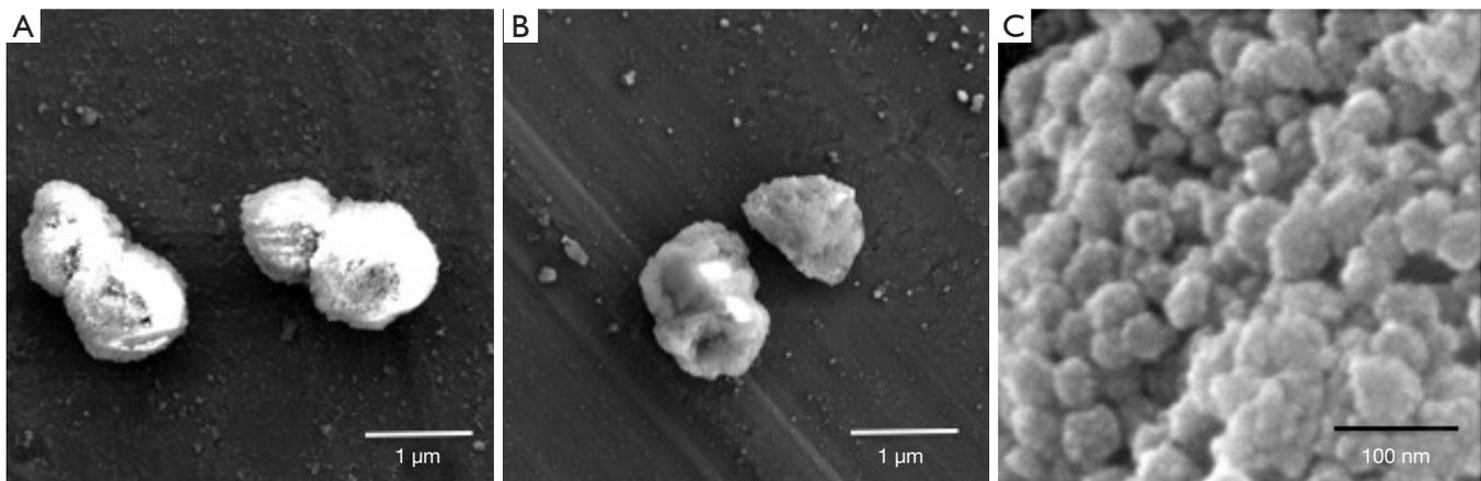
**Figure 2** SEM images of  $\text{Ca}^{2+}$ @MSNs (A),  $\text{PO}_4^{3-}$ @MSNs (B) and  $\text{Ca}^{2+}/\text{PO}_4^{3-}$ @MSNs (C). The surface of the  $\text{Ca}^{2+}$ @MSNs/ $\text{PO}_4^{3-}$ @MSNs was relatively rough.  $\text{Ca}^{2+}/\text{PO}_4^{3-}$ @MSNs showed a significant decrease in particle diameter due to the ion release. MSNs, mesoporous silica nanoparticles.
