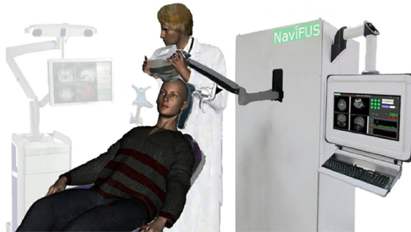
Figure 1 Schematic diagram of NaviFUS. The NaviFUS is a focused ultrasound phased array system in conjunction with clinically available neuronavigation to intraoperatively guide FUS energy deposit in the deep brain targeting position. A patient is fixed semi-rigidly without headpin system. A hand-held probe is connected to the power generator and working station. A doctor can steer the probe for precise transcranial targeted region under neuronavigation guidance. The whole procedure can be completed in one hour.
