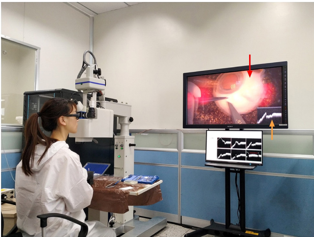
Figure S1 The microscope integrated optical coherence tomography (MIOCT) and external 3D head-up visualization system. The MIOCT images (yellow arrow) and surgical microscopic images (red arrow) are simultaneously projected on the external 3D head up display.
