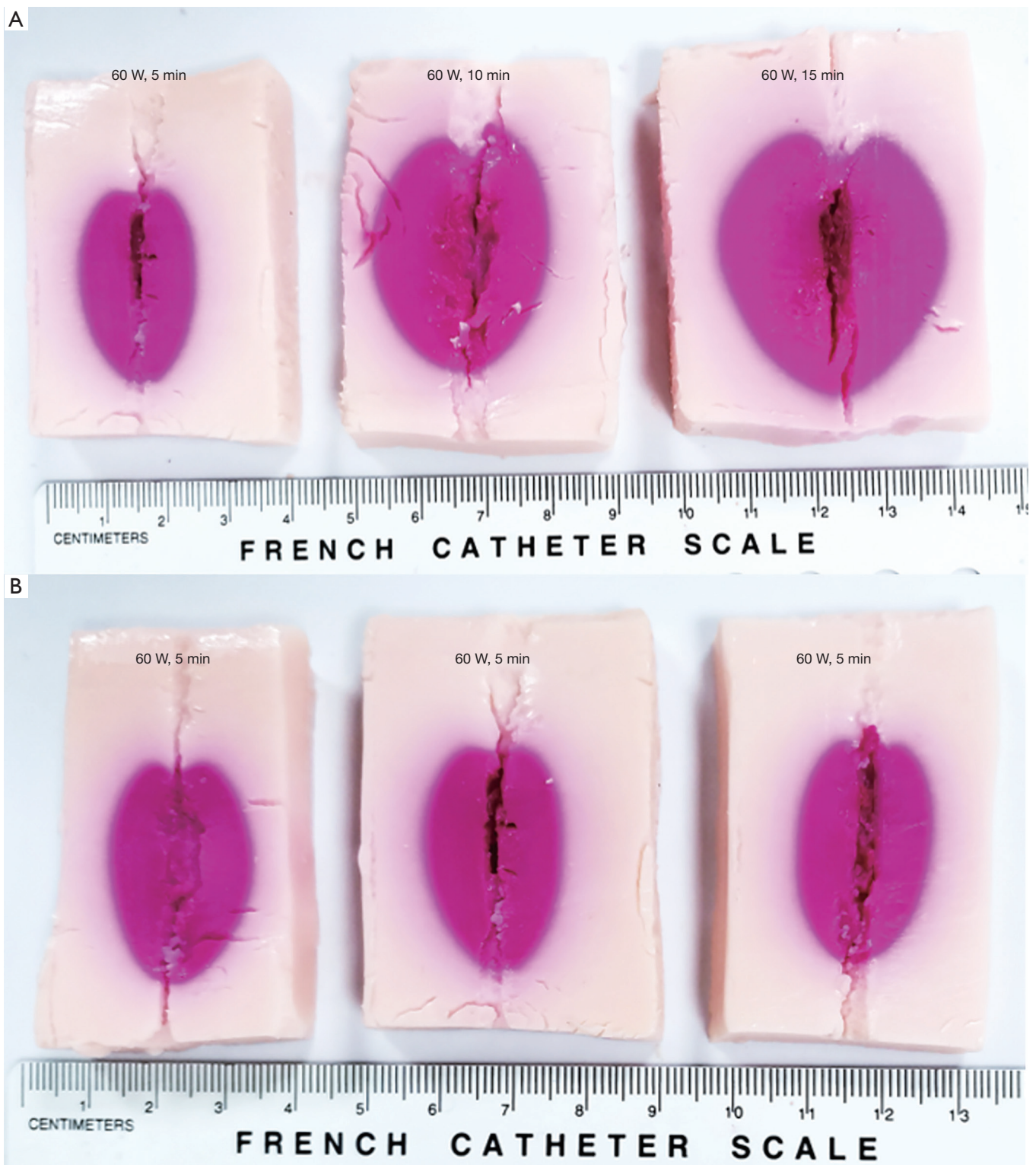
Figure 2 The gross specimen of the phantom model after MWA. (A) Phantom samples were ablated with 60 W at a different time; (B) phantom samples were ablated with the same power and time at 60 W, 5 minutes.
