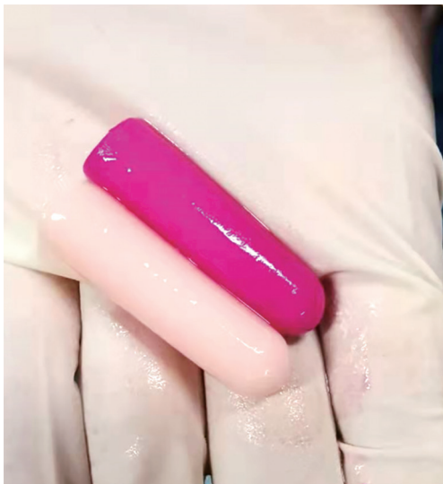
Figure 1 The color differences of phantom samples with (magenta one) and without (cream white one) hot water bath.
