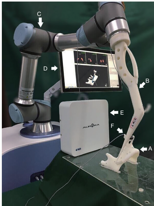
Figure 4 Model experiment of our maxillofacial surgical robotic system (MSRS). (A: mandible model mounted with navigation splint; B: template; C: robot; D: computer; E: EM generator; F: EM sensor).
